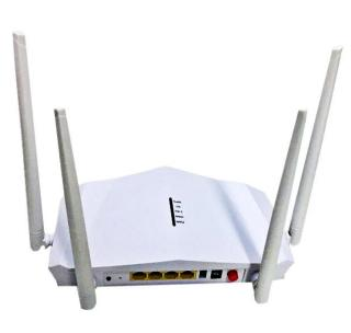
WR3000-18 adopts the MTK MT7561DU scheme. Downlink provides 3 GE interfaces, uplink provides 1 GE interface, 1 USB3.0, 2x2 dual-frequency wireless combined network speed up to 1800Mbps. The wireless is based on 802.11ax (Wi-Fi6) technology, and compared to traditional Wi-Fi, it combines OFDMA and MU-MIMO technologies to effectively allocate channels. with lower while latency communicating with multiple devices, and multi-device transmission is theoretically 4 times faster.
